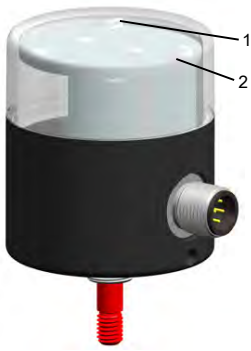
Fig. 7: High-visibility LED (1) / magnetic sensor for in-situ initialisation (2)
