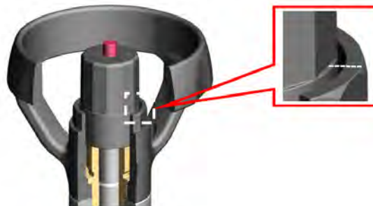
Fig. 13: Locating sleeve flush with upper edge of handwheel
