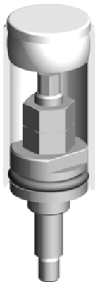
Fig. 40: Closed-position travel stop
