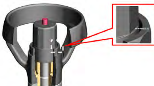
Fig. 12: Locating sleeve flush with upper edge of handwheel
