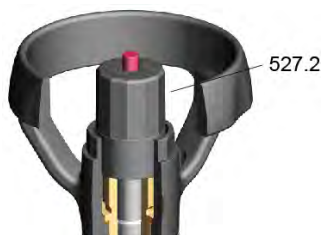
Fig. 11: Setting the open-position travel stop
