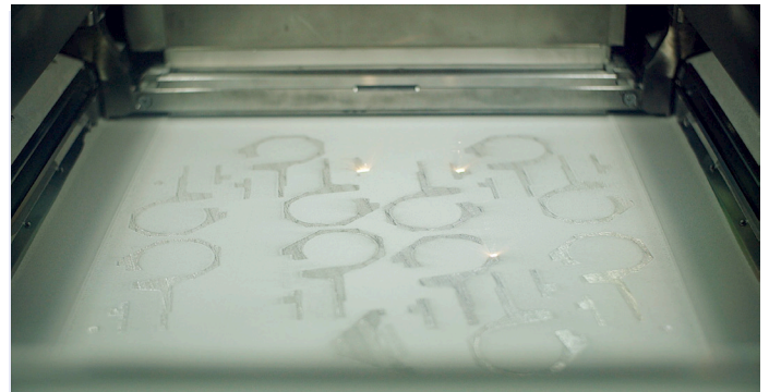
2. Additive manufacturing using the powder bed fusion process
